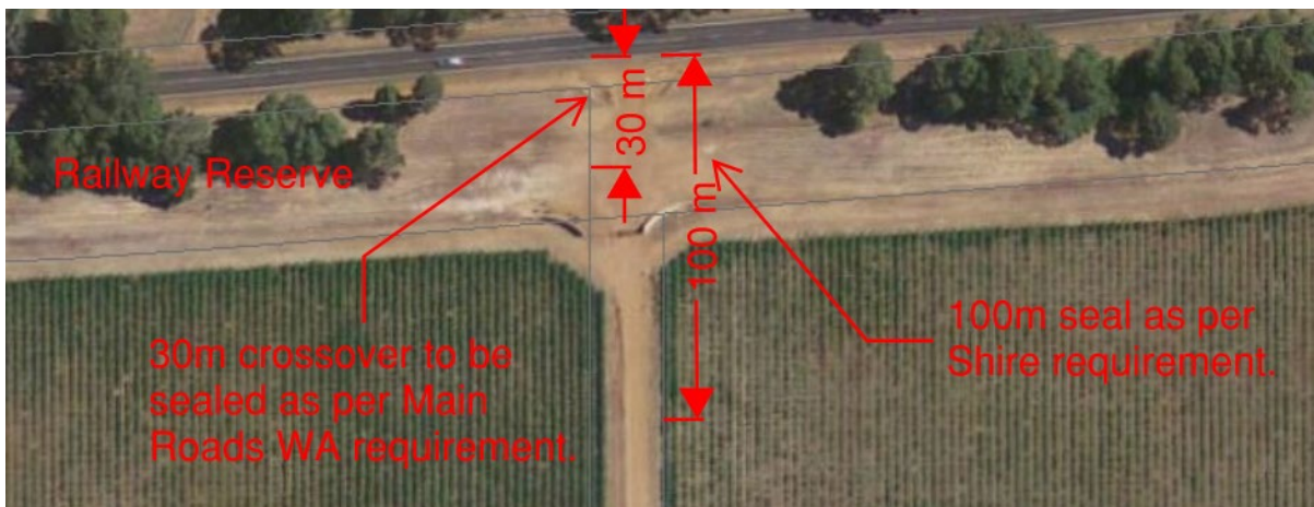
Figure 6 - Bitumen seal of the first 100m of access road.
